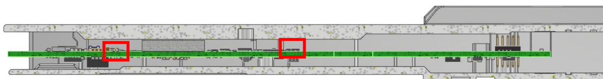
Figure 6: ML4064-AL6R-224 Temperature sensors location
